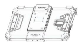
3. With home buttons to the right, fit Galaxy Tab Active2 bottom into case, as shown. Snap top corners into place. (E,F)
