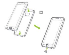
2. Remove the Removable Accent Plate from the back of the uniVERSE Case. Align the case with the uniVERSE Case Adaptor and slide down until you hear a click indicating it is in place. (B)
