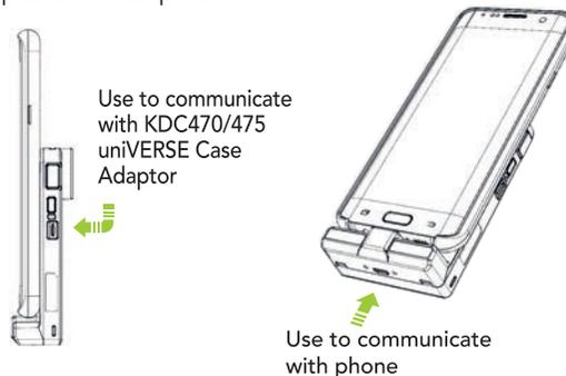
\*Both USB ports support simultaneous charging of KDC470/475 and phone.
