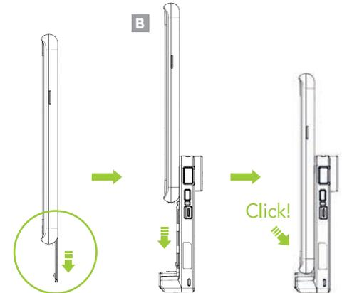
4. Inspect the connection between the uniVERSE Case Adaptor and previously installed OTG USB Connect Head. To test the connection, attempt to charge your device via USB or Charging Cradle - the device will begin charging if the connection is successful. (C)
