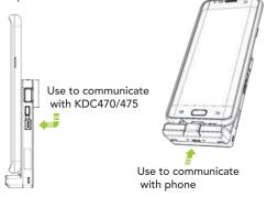
\*Both USB ports support KDC470/475 and phone simultaneous charging.
