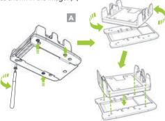
2. To remove the KDC180 from the uniVERSE Adaptor, pull up while pressing the buttons on both sides of the uniVERSE Adaptor cap. (D)
